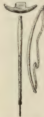
ESKIMO BOW DRILL SHOWING PARTS
